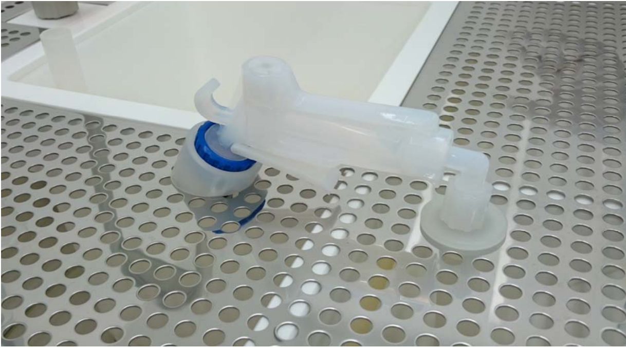
Example of a possible way of embedding the DIW gun or N2 gun in the surface.
